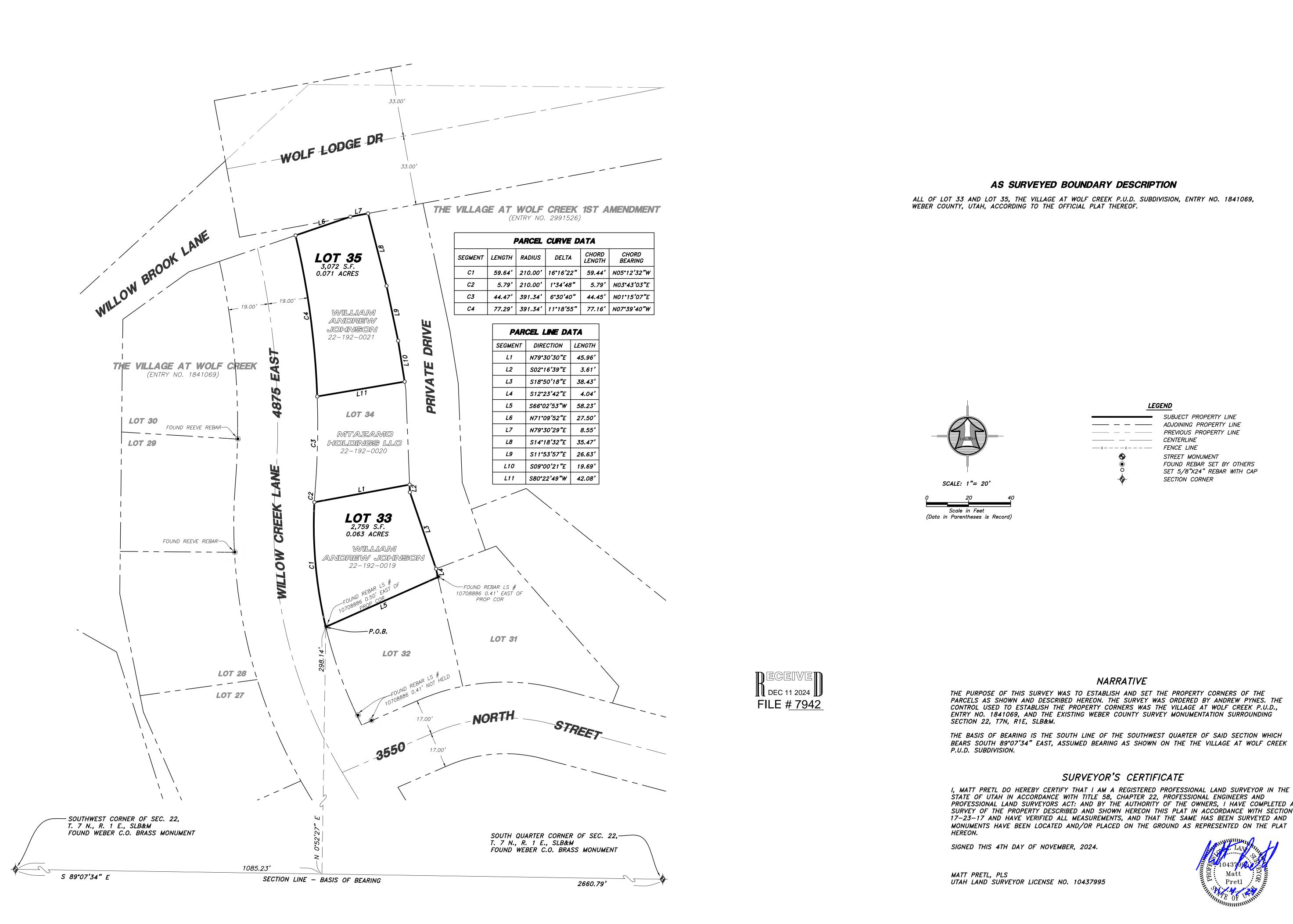
THE PURPOSE OF THIS SURVEY WAS TO ESTABLISH AND SET THE PROPERTY CORNERS OF THE PARCELS AS SHOWN AND DESCRIBED HEREON. THE SURVEY WAS ORDERED BY ANDREW PYNES. THE CONTROL USED TO ESTABLISH THE PROPERTY CORNERS WAS THE VILLAGE AT WOLF CREEK P.U.D., ENTRY NO. 1841069, AND THE EXISTING WEBER COUNTY SURVEY MONUMENTATION SURROUNDING
