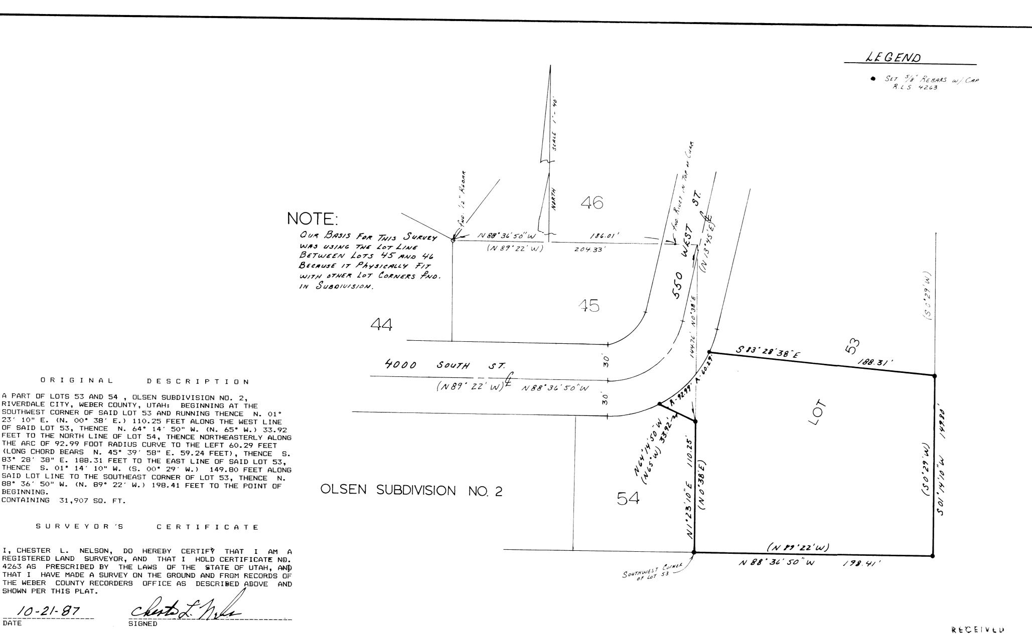
THE PURPOSE OF THIS SURVEY WAS TO SURVEY PART OF A LOT REQUESTED BY THE BUYER, LOCATED IN WEBER COUNTY, UTAH. THE SUBDIVISION BASIS OF BEARINGS WAS N. 87° 22' W. ALONG THE SOUTH LINE OF THE SOUTHEAST QUARTER OF SECTION 6, TOWNSHIP 5 NORTH, RANGE 1 WEST, S.L.B. & M., THE BASIS OF BEARINGS HAS BEEN ROTATED TO THE STATE PLANE GRID BEARINGS OF N. 88° 36' 50" W. ALONG THE SOUTH LINE OF SAID SOUTHEAST QUARTER.
