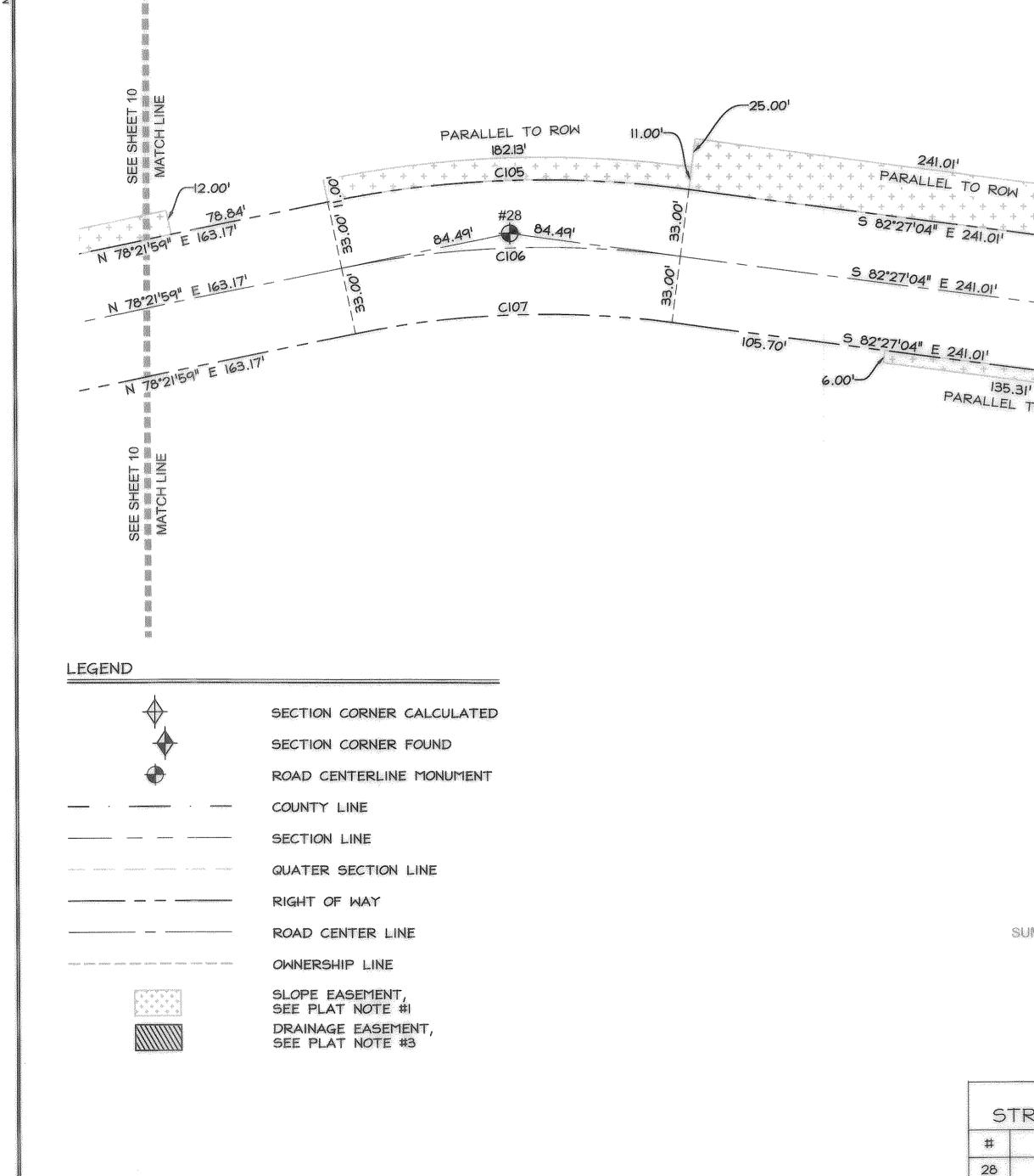
ALL SLOPE EASEMENTS ARE PARALLEL TO R.O.W.
