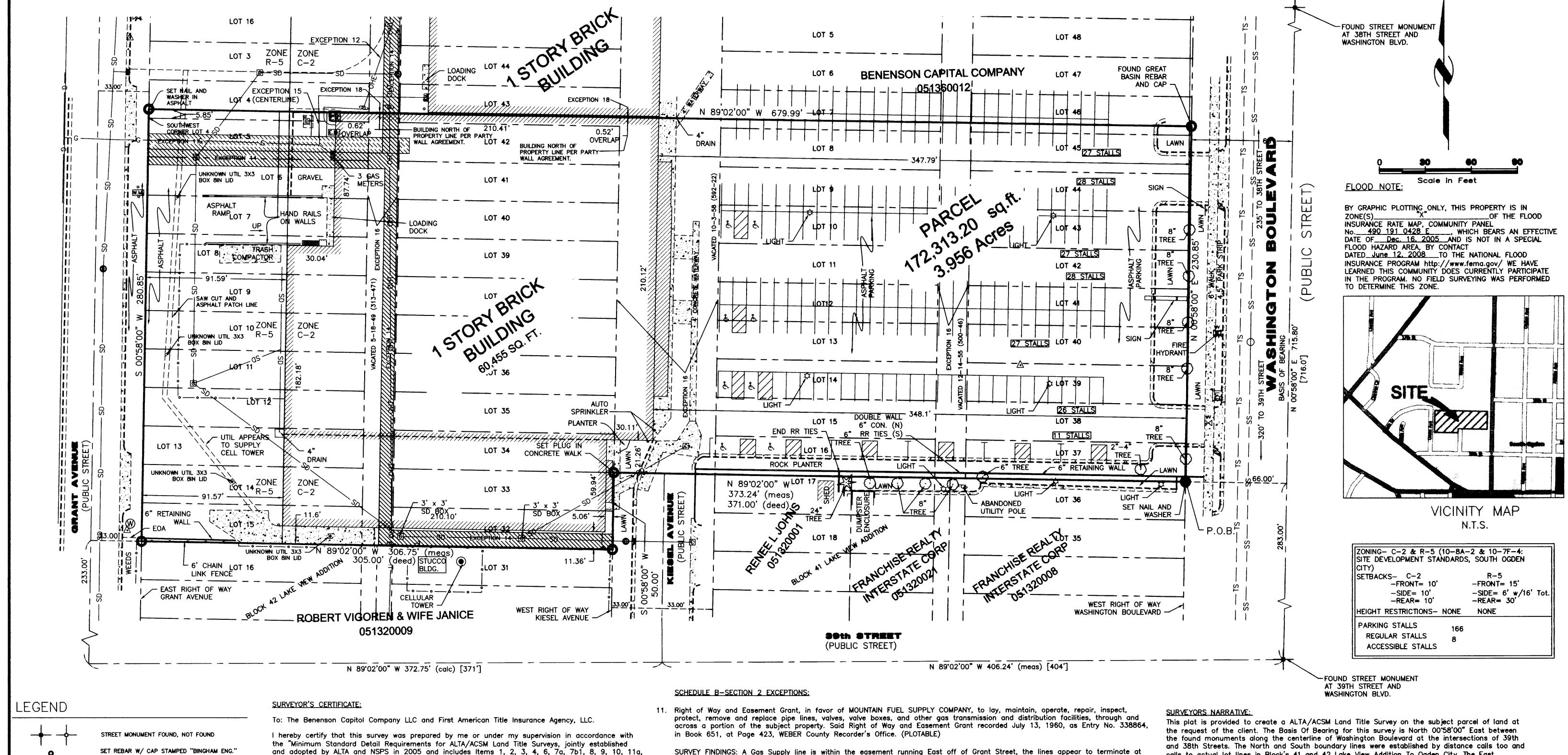
SET REBAR W/ CAP STAMPED "BINGHAM ENG." (UNLESS OTHERWISE NOTED) HIM W HIM EXISTING FIRE DEPT. CONNECTION, HYDRANT, WATER VALVE, METER, MAN HOLE E or ← EXISTING ELECTRIC BOX, UTILITY POLE, GUY WIRE **S** EXISTING SEWER MANHOLE G.M. EXISTING GAS METER EXISTING STREET LIGHT  $\dot{\mathbf{x}}$ EXISTING CATCH BASIN EXISTING SIGN EXISTING BOLLARD PROPERTY BOUNDARY LINE
