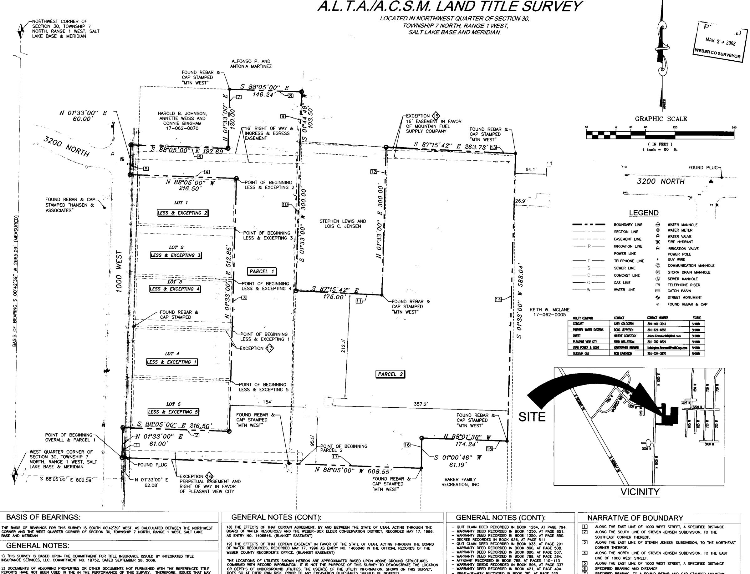
THE BASIS OF BEARINGS FOR THIS SURVEY IS SOUTH 00'42'39" WEST, AS CALCULATED BETWEEN THE NORTHWEST CORNER AND THE WEST QUARTER CORNER OF SECTION 30, TOWNSHIP 7 NORTH, RANGE 1 WEST, SALT LAKE
